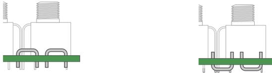
For summing configuration, insert resistors of your choice in the jumper locations. This option has NOT been evaluated by f(h) and will affect the signal levels, as you are adding resistance to the input and output path. Possible mounting orientations are shown below. In the latter examples, make sure the leads do not make contact with the faceplate.
