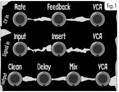
The jacks are grouped by the type and direction (into or out of the module) of the relevant signal. The VCA jacks are just labeled "VCA", as the function of each is already described by what row they are in.
