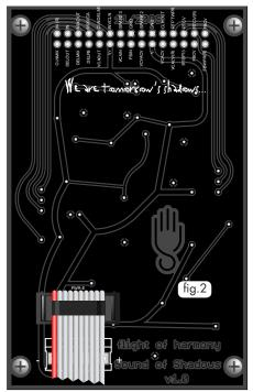
Power: The power connector header is a 2x5 shrouded box header which accepts the standard Doepfer power cable. This header style is polarized, meaning the connector can only be inserted one way, to prevent connecting the power backwards and damaging the unit. THIS ASSUMES THAT YOU ARE USING THE EITHER THE SUPPLIED CABLE OR ONE MANUFACTURED BY DOEPFER! Looking at the rear of the module, the negative supply (red stripe) is on the left, positive supply is on the right (see fig. 2).
